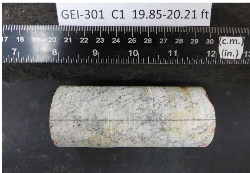
After cutting and grinding
