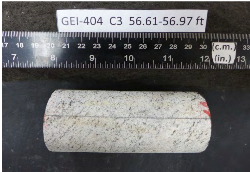
After cutting and grinding
