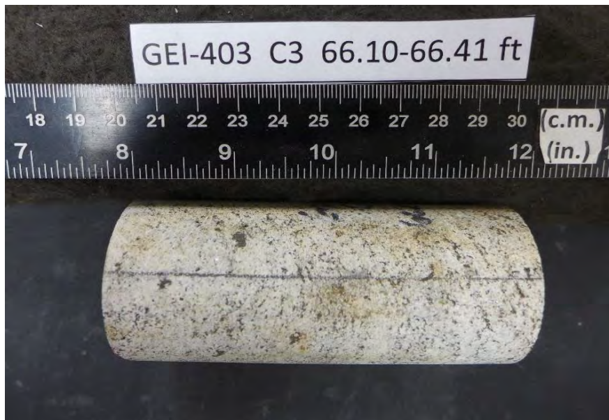
After cutting and grinding
