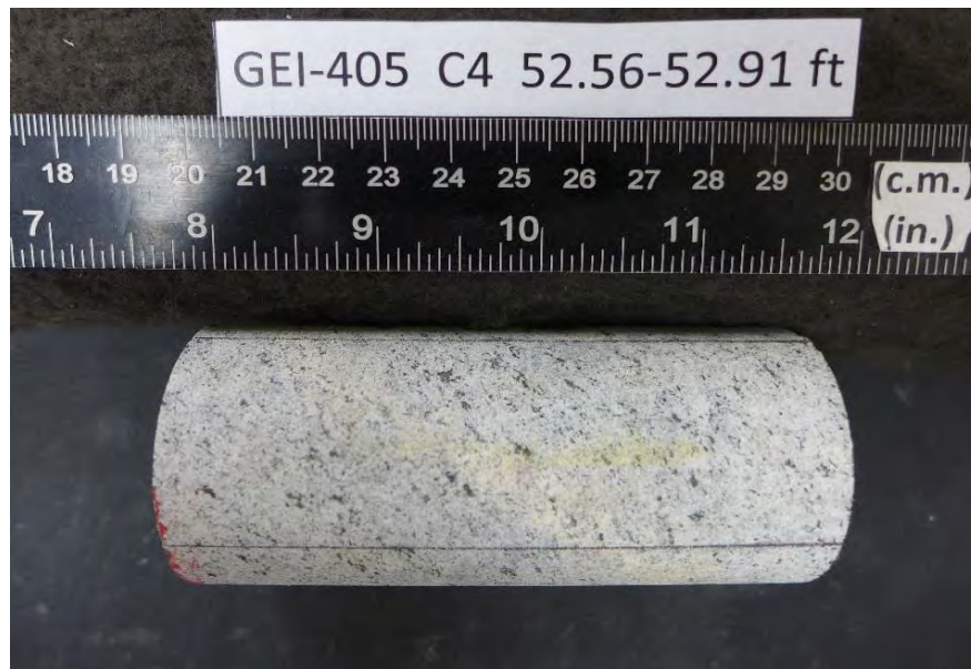
After cutting and grinding
