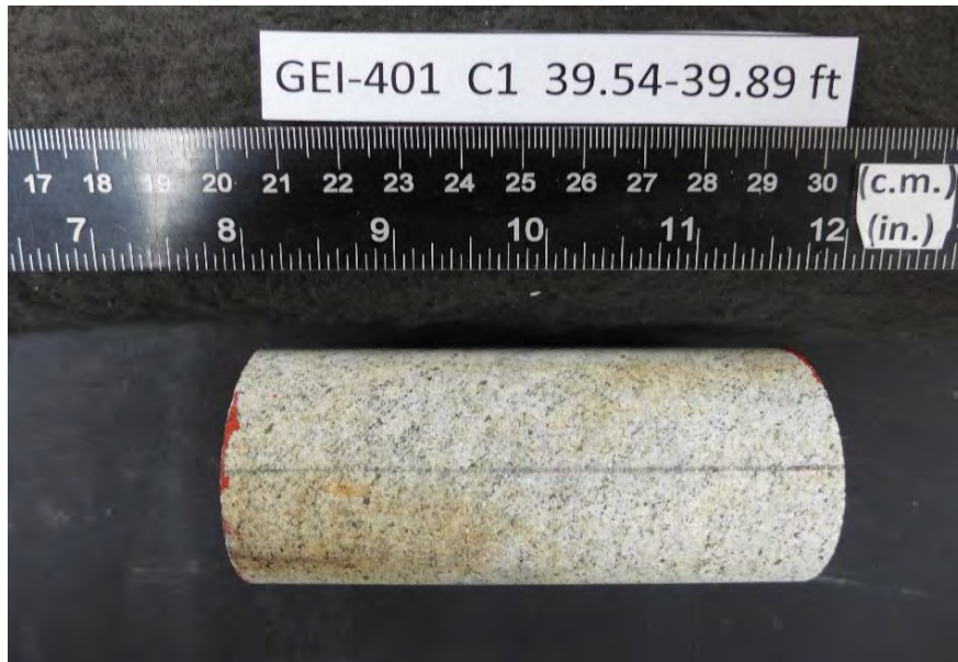
After cutting and grinding
