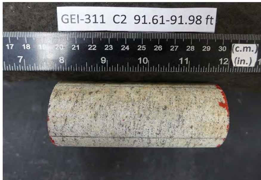
After cutting and grinding
